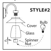
**STYLE#2** - Remove spinner nut from socket. Position cover and glass on lamp and secure with spinner nut. Install specified bulb type and wattage (not included).
